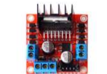
Fig 5: L298N Motor Driver
